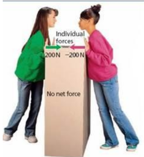
Balanced Forces in Opposite Directions When two equal forces act in opposite directions, they cancel each other out. The box doesn't move.
